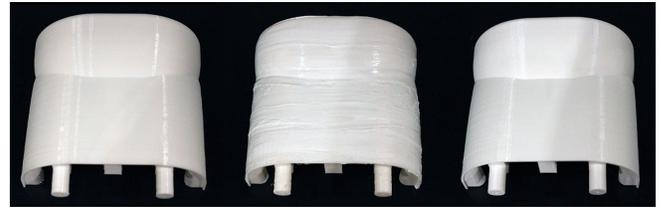
Figure 2. The three materials used for the torso part of the robot are Polyurethane (PU) (left), Silicone-coated Acrylonitrile Butadiene Styrene (middle), and Acrylonitrile Butadiene Styrene (ABS) (right).
